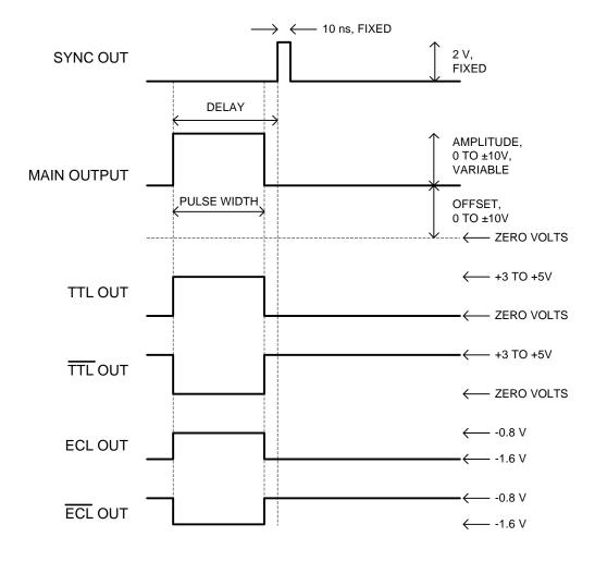
The next figure illustrates the relationship between the signals when an external TTL-level trigger is used (i.e., the REPETITION RATE switch is set to "EXT"), assuming that the delay mode is set to "MAIN OUT DELAYED":
