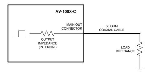
However, to obtain output amplitudes greater than  $\pm 5V$ , the  $\pm 10V$  ranges must be used, and the output impedance will be  $2\Omega$ . This is slightly less ideal, but good waveforms will still be obtained since the transmission line is still properly terminated on one end (the load end) with  $50\Omega$ .
