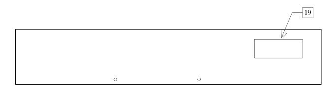
19. <u>AC POWER INPUT</u>. A three-pronged recessed male connector is provided on the back panel for AC power connection to the instrument. Also contained in this assembly is a slow blow fuse and a removable card that can be removed and repositioned to switch between 120V AC in and 240V AC in.
