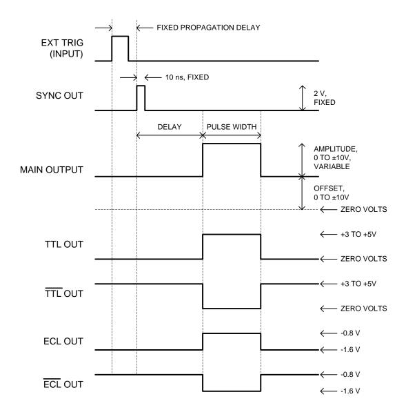
As before, if the delay mode is set to "MAIN OUT ADVANCED", the order of the SYNC and OUT pulses is reversed.
